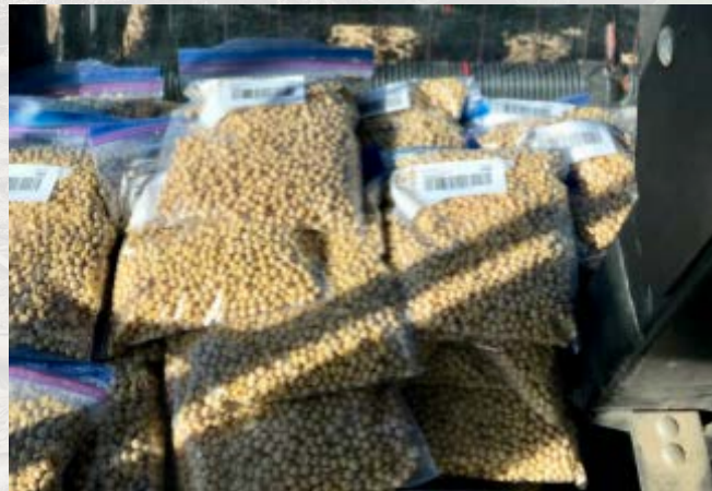
Figure 4. Soybean grain samples collected during FIRST harvest operations for later analysis at the University of Minnesota. Samples are stored in plastic bags for up to several weeks before being measured for moisture, some dried, and scanned with benchtop NIRS instruments to estimate protein and oil content.
