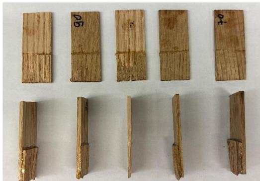
**Figure 16.** Adhesive failure of CSBO\_TAA (2.5 equiv.) under optimized conditions.
