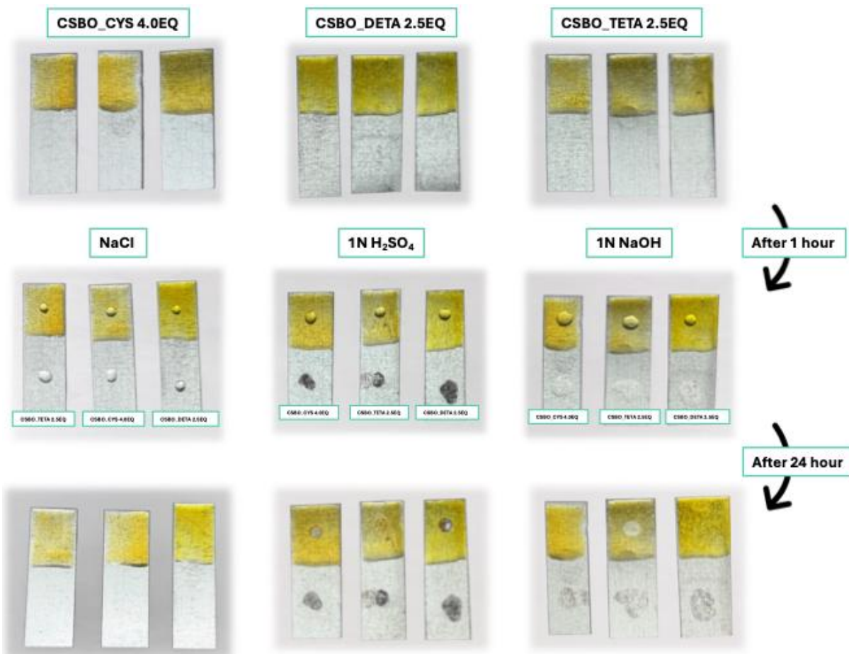
Figure 3. Chemical resistance test of uncoated and NIPU-coated stainless-steel coupons in NaCl (sat. solution), 1N H 2 SO 4 , and 1N NaOH solution.
